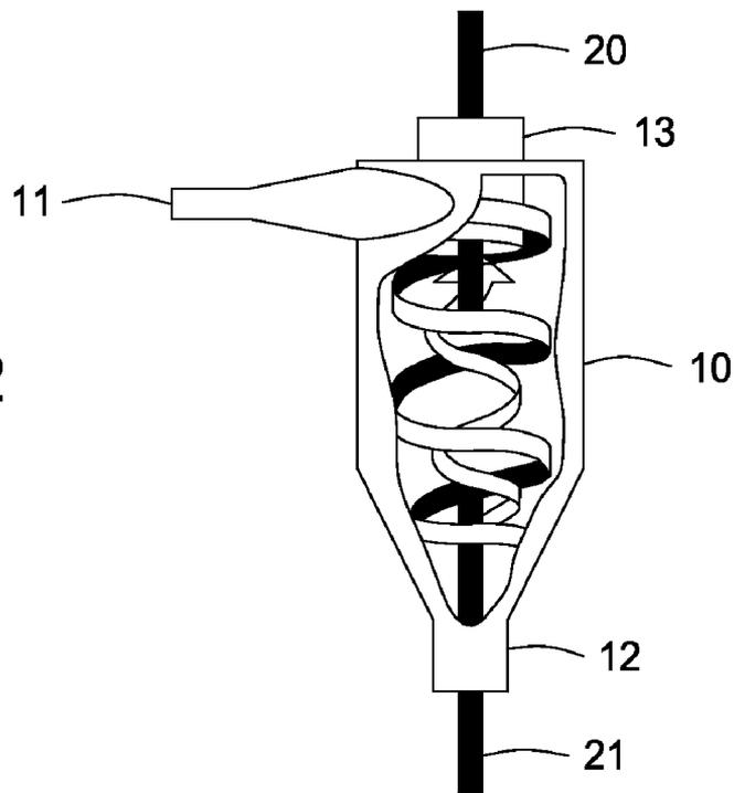
Carbon Arc in Cyclone separator
