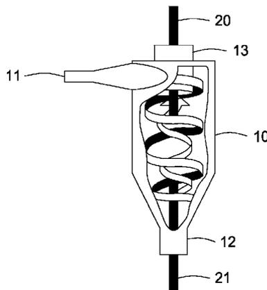
Carbon Arc in Cyclone separator
