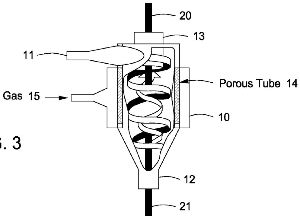
Carbon Arc in Gas-Sparged Hydrocyclone
